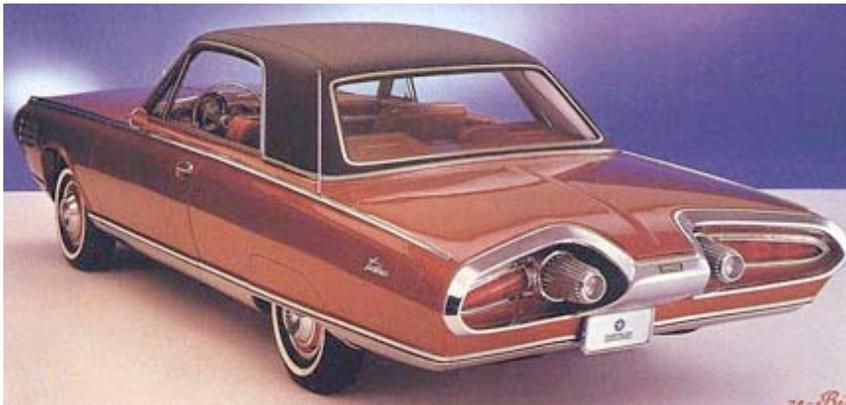
Chrysler Turbine Cars were automobiles powered by gas turbine engines that the Chrysler Corporation assembled in a small plant in Detroit, Michigan in 1963, for use in the only consumer test of gas turbine-powered cars. The bodies and interiors were crafted by Ghia in Italy. Of the 55 units built, most were scrapped at the end of a trial period, with only 9 remaining in museums and private collections. It was the high point of
